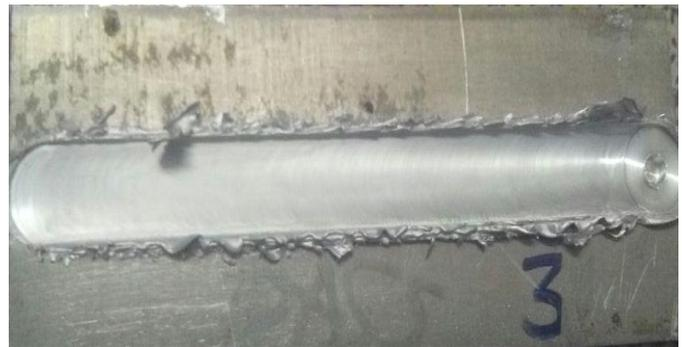
Figure 2(d): Triple pass on the fourth Al workpiece with SiC
